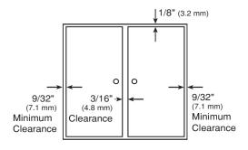
Note: Some minimal clearance may be required for paint and/or weatherstripping.
